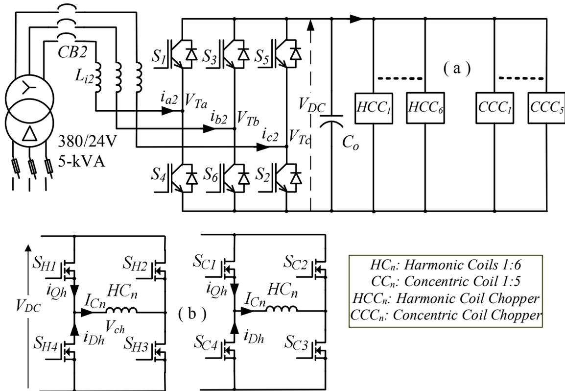
Fig.2 Power Circuits of Harmonic and Concentric Coils
