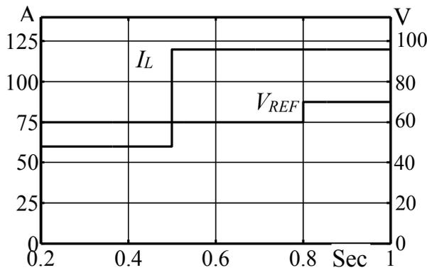
Fig.5a Step in Voltage Reference and Current disturbance for VSC
