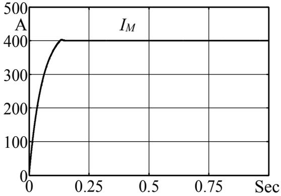
Fig.4a Step Response of CSC Controller Feeding the Main Coil
