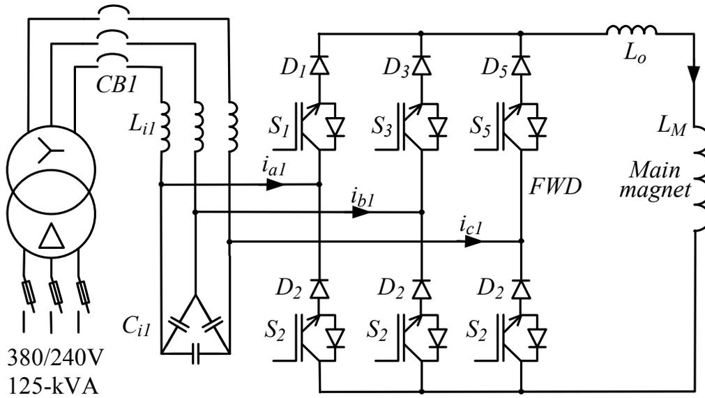
Fig.2 PWM Unity Power Factor Current Source Converter to Supply Main Magnet Coil
