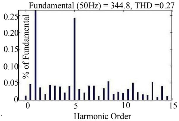
Fig.4d Harmonic Spectrum of CSC Supply Current
