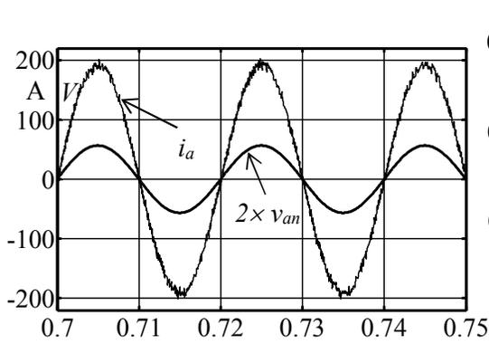
Fig.5e Supply Current and Voltage Waveforms Under heavy loading
