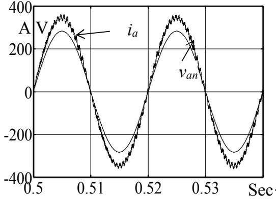
Fig.4c Supply Current and Voltage Waveforms of The CSC
