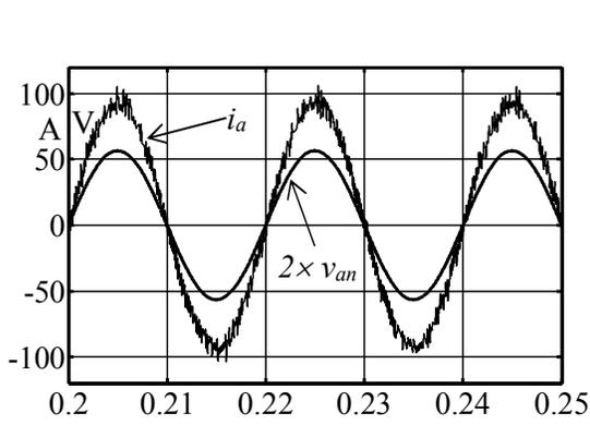
Fig.5c Supply Current and Voltage Waveforms Under light loading
