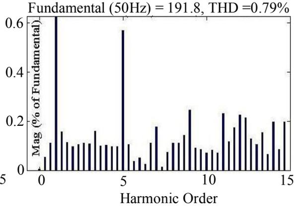
Fig.5f Harmonic Spectrum of Supply Current shown in Fig.5e
