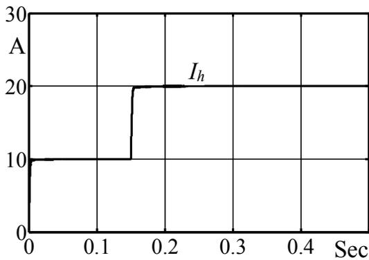
Fig.6a Response of Chopper Current Controller Feeding the Harmonic Coil
