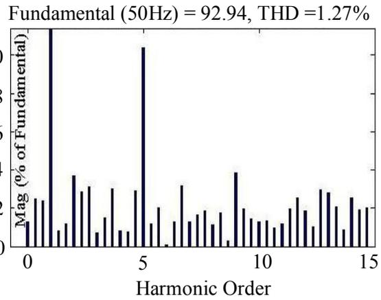
Fig.5d Harmonic Spectrum of Supply Current shown in Fig.5c
