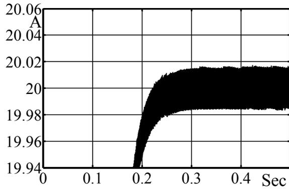
Fig.6b Expanded View of Fig.7a to show the Ripple Content in Current
